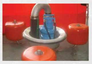
A light weight high capacity weir skimmer with a high performance helical screw pump, equipped with self-adjusting weir lip and 3 detachable HDPE outrigger floats for increased stability in waves.
