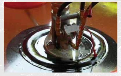
2 sizes of the helical screw pumps that can handle all types of oils and with the precision made pump housing made of heat treated aluminium and the stainless steel impeller, it will serve your pumping needs for many years. The oil transfer pump can easily be detached by loosening 3 bolts and may be used as a submersible oil transfer pump. The minimum required power to operate the skimmer is the 7.3 kW (low capacity) and at full capacity 100 m3/h 25 kW power is recommended.
