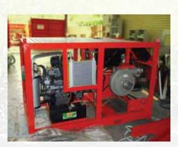
Diesel driven power pack from 3 kW to 55 kW for operation of a wide range of oil spill response equipment.
