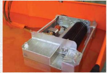
Disc/brush combination skimmers are designed for operation in all types of oil. In light oils discs are used and for oils with higher viscosity you change to brushes. The quick shift feature of the disc/brush bank ensures minimal stoppage time.
