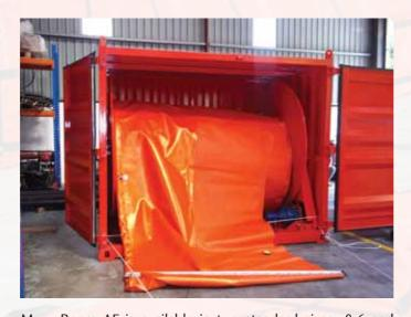
My – Boom AF is available in two standard sizes: 0.6 and 0.75 meter inflated overall width. It is lightweight and quick to deploy and can be pulled very rapidly into the water, either from a container, from a boom reel or right from the beach. The average deployment time is 12 to 20 minutes for 200 meters, depending on the experience of the operators and the accessories included in the system.
